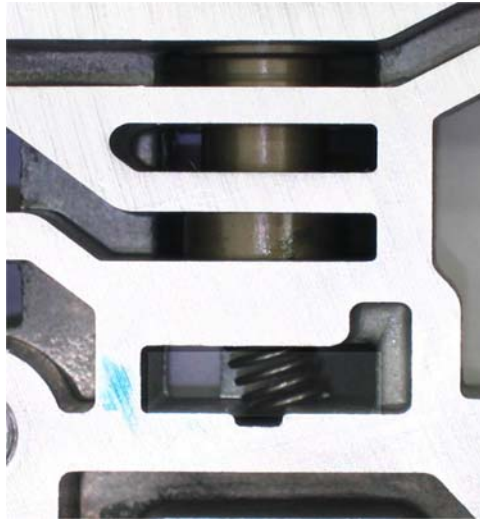
Checking CPC Valves
